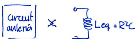
$$\left. \begin{array}{l} \text{Si } C = 1 \mu F \\ R = 1 k\Omega \end{array} \right\} L_{eq} = 1 H$$
